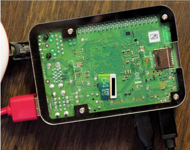
Now that the Pi is assembled and the card is installed, we're ready to go. Well, almost. It's pretty easy to miss the SD slot, and the card gets stuck between the Pi and the case. Shake it until it comes out again. Yes, that's a 64GB card whereas I'm using a 32GB card for the project. There's a lot of bad continuity in this presentation. Spot them all and win a prize! (Not really.)
